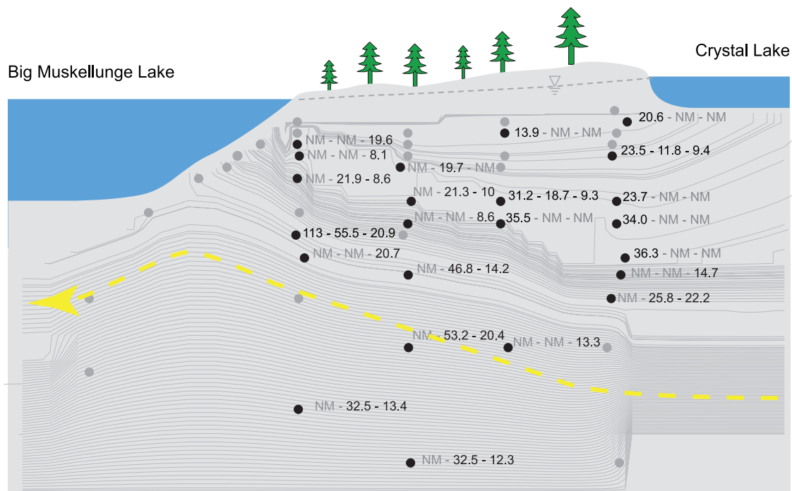
Figure 17. Pathlines based on hydraulic conductivity field estimated using head, \delta^{18}\text{O} , and tritium data. The yellow dashed line is representative of the general flow path at depth. The numbers next to the dots indicate tritium concentrations in tritium units (TU). The labeling scheme is further described in Figure 14. Figure not to scale.
