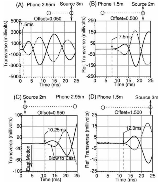
FIG. 13. Superposition of alternative *SH*-wave polarizations as recorded on transverse geophones. *SH*-wave arrivals are picked at the point where the traces depart. Different offsets are shown: (a) 0.05 m, (b) 0.5 m, (c) 0.95 m, (d) 1.5 m.
