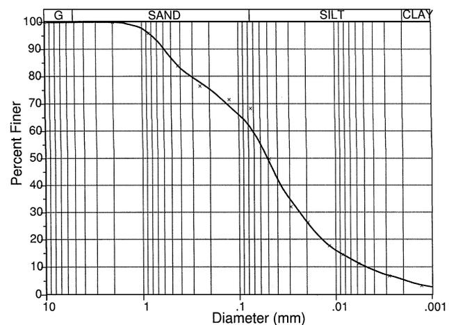
FIG. 4. The standard grain-size distribution. The soil is a sandy silt (ML, unified system).
