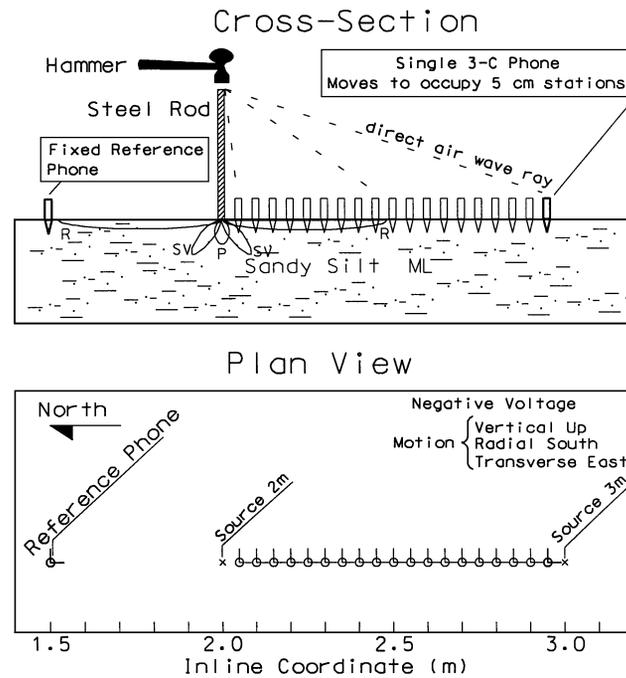
FIG. 3. Experimental geometry in cross-section and plan view. Only two 3C geophones were used. The reference geophone remained stationary at coordinate 1.5 m. The moving geophone traveled between the two source positions. Common source position gathers yield reverse profiles.
