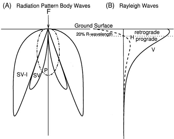
FIG. A-1. (a) Approximate directivity patterns for far-field *P*- and *SV*-waves in an elastic half-space, vertical point-source function. (b) Typical vertical and horizontal displacement eigenfunctions for a Rayleigh wave (after Miller and Pursey, 1954).
