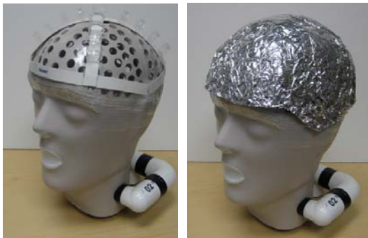
Figure 2. Illustration of thermal manikin wearing the spacer harness and reflective helmet.
