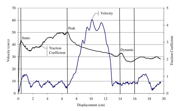
Figure 16: Traction coefficient and shoe velocity for a representative trial
