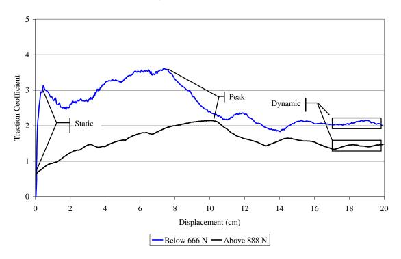
Figure 15: Representative Traction curves below 666 N and above 888 N
