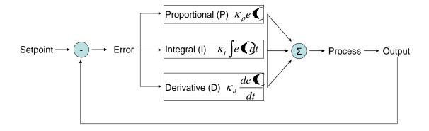
Figure 11: Block diagram of a generic PID controller
