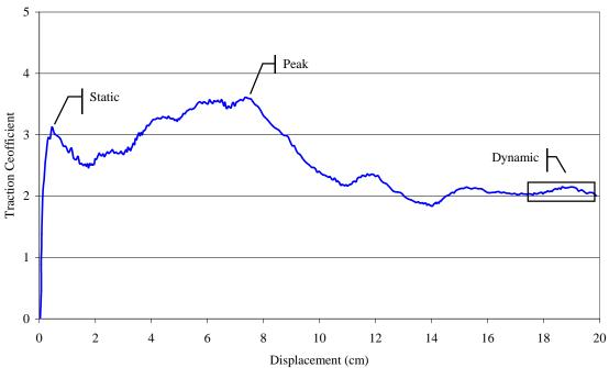
Figure 12: Static, Peak, and Dynamic traction variables defined
