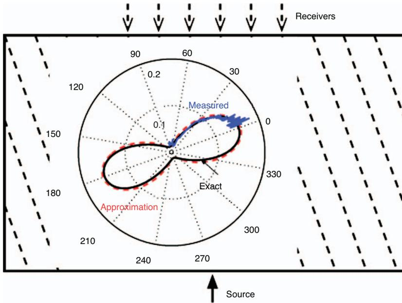
Figure 6. Polar plot of the attenuation coefficient against the background of our physical model. The estimated function  $\mathcal{A}(\theta)$  from Figure 5 (blue curve) was used to find the best-fit attenuation coefficient from the Christoffel equation 1 (black) and approximate equation 2 (dashed). The numbers on the perimeter indicate the phase angle with the symmetry axis.
