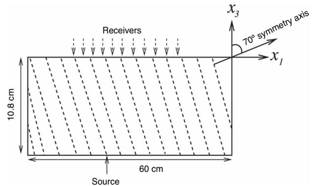
Figure 1. Physical model of a TI layer with the symmetry axis tilted at  $70^\circ$  (from Dewangan et al., 2006). The transmitted wavefield is excited by an ultrasonic contact transducer at the bottom of the model and recorded by a laser vibrometer.
