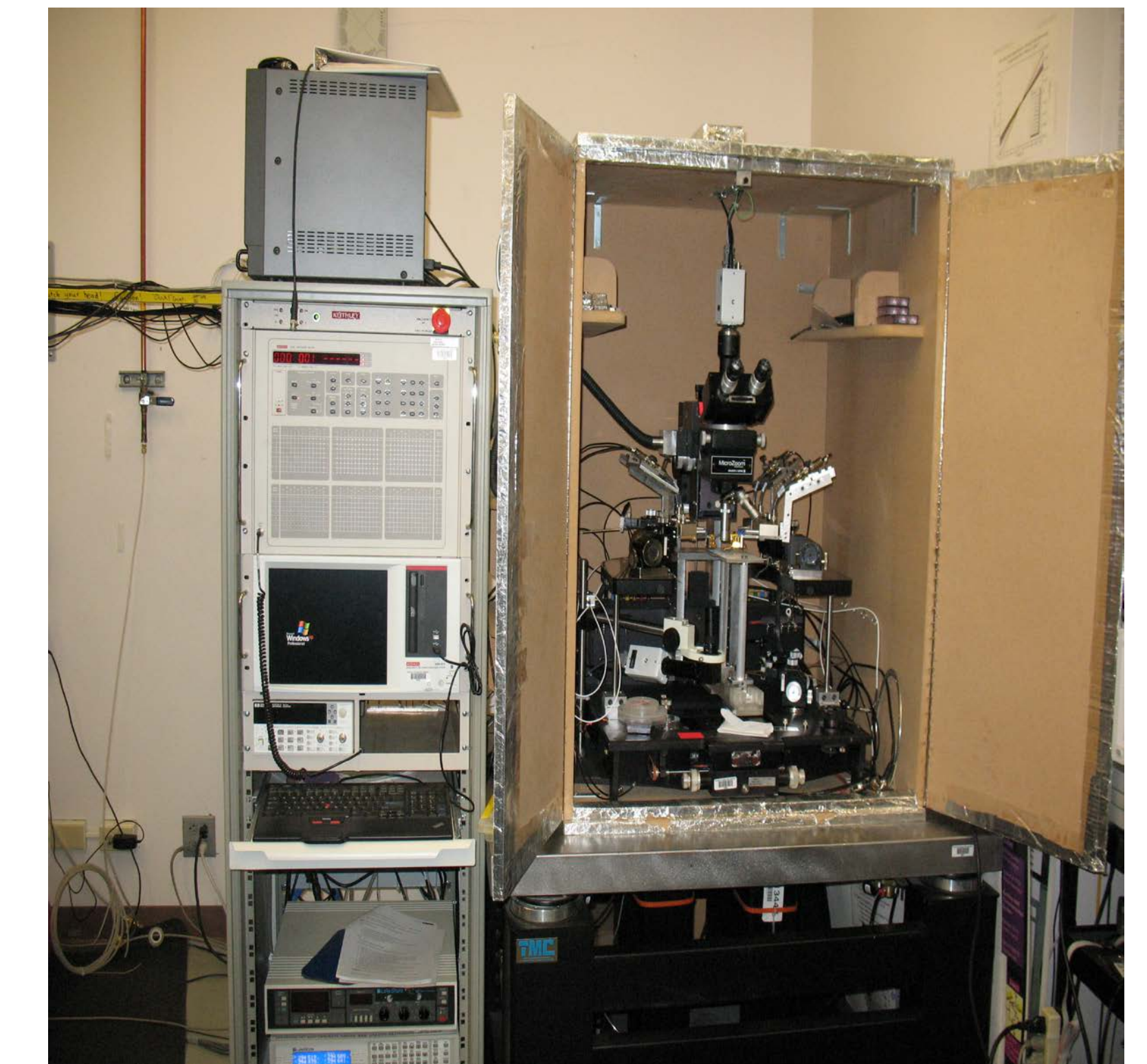
Fig. 7 Keithly characterization system used to perform voltage sweep test on devices
