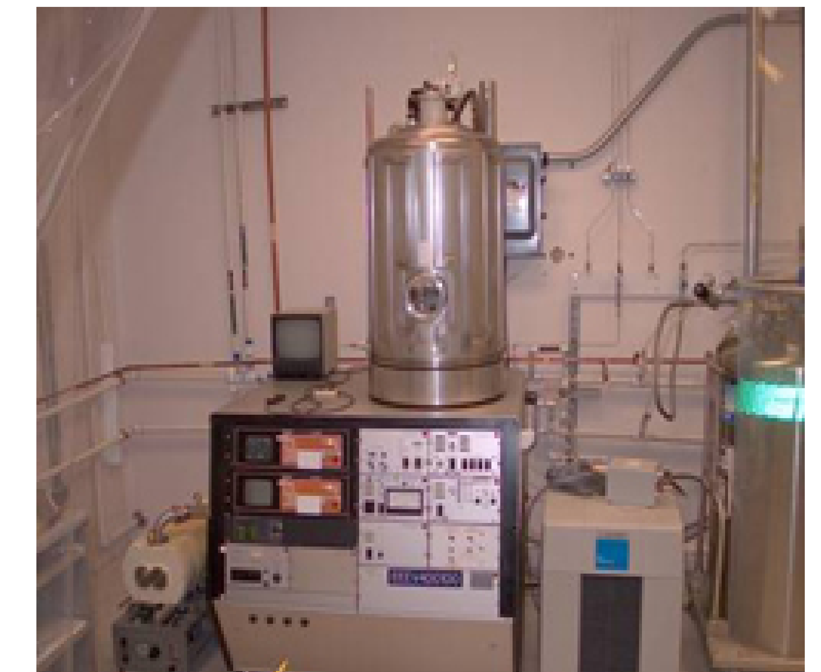
Fig. 8 Thermal evaporation station that will be used in future fullerene deposition techniques
