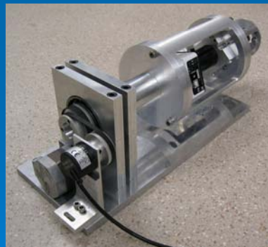
Figure 4 (right): Shown is the stepper motor and the rotational encoder mounted on the rotational device. The motor is geared down by 5:1 while the encoder is directly connected to the device's shaft. Camera and optics can be seen in the back of the device
