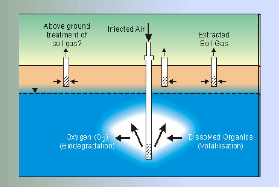
An injection well pumps air into the contaminated ground water
