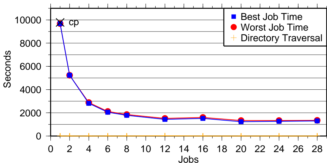
Figure 3.12: Best and Worst Bpct Jobs on Icestorm Copying “Few Large Files” Set of 7.24. The cp time on one node for this data set is 9776 seconds. The results are listed in Table 3.14 and graphed in Figure 3.12.
