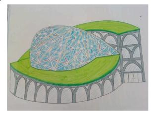
roofed structures surrounding the gem will also have a glass and steel construction, with an arched design for superior support of the grass roof. The roof will be covered in a special grass plant that requires maintenance once a year, maintains color well, and is almost self-sufficient for water. This provides a natural insulation for the building, lowering energy costs for the building.
