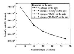
Fig. 6. Drain current as a function of channel length. Note at this scale the modulation is not readily apparent. (tox=200?,  $N_{SUB}=10^{15}/cm^3$ )
