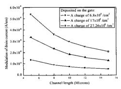
Fig. 7. Modulation of drain current as a function of channel length. (tox=200 ? ,  $N_{SUB}$ =10<sup>15</sup>/cm³)
