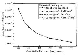
Fig. 4. Drain current as a function of gate oxide thickness. Note at this scale the modulation is not readily apparent. (L=  $10~\mu m, N_{SUB}=10^{15}/cm^3$ )
